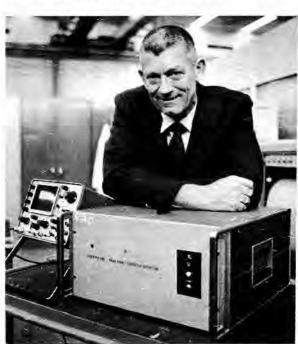
SYSTEM FOR DETECTING airborne particles in a laminar air flow clean room is displayed by inventor Bill Neitzel (9225). Instant read-out is available on a digital counter, a digital recorder, and an audible indicator.
